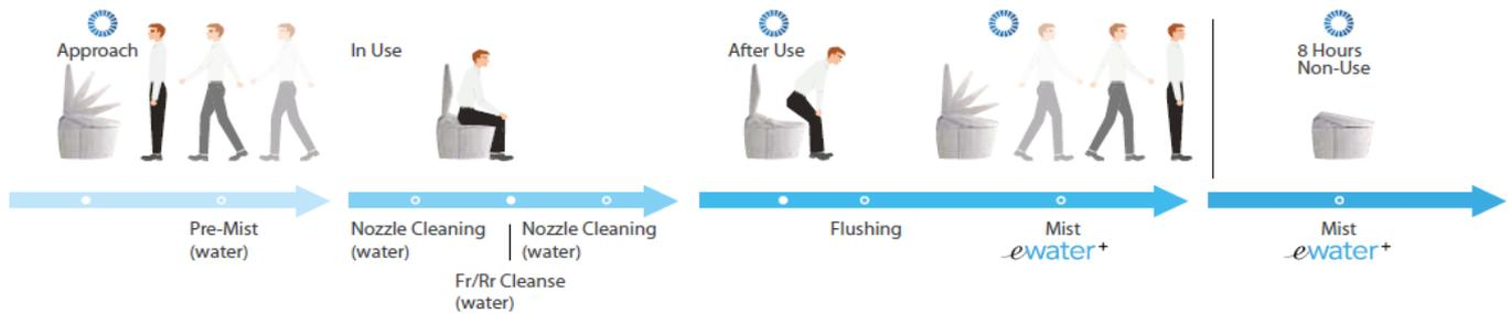
The wand system is a technology that utilises water to provide personal cleaning, ensuring a whole new level of hygiene. Warm water is, after all, much more effective at cleaning than toilet paper. The position, temperature and pressure of the water jet can all be adjusted. After use, the wand cleans itself automatically.
